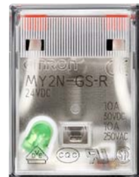
Relay with DC Coil (LED: Green)
